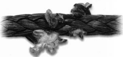
Rope displays two adjacent cut strands-- rope should be replaced.
